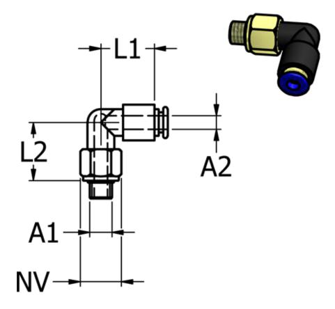
Ext. hose diameter A2 = 3 mm L1 = 12 L2 = 16.5 NV = 10 Thread A! = M6
